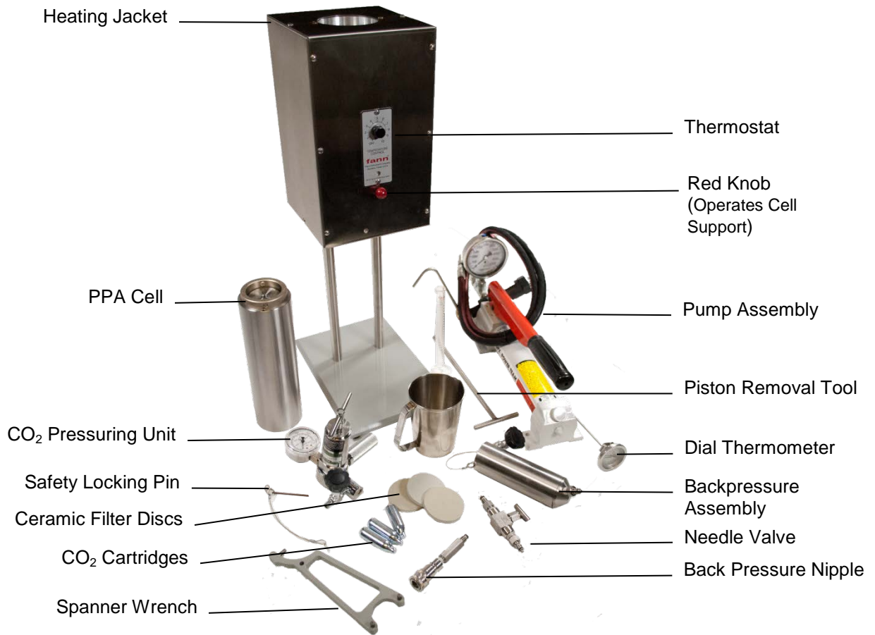
Figure 3-1 Permeability Plugging Apparatus Assembly
